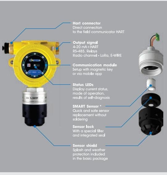
DGS ERIS 210 is the reliable explosion-proof gas detector for flammable, toxic gases and oxygen monitoring hazardous areas - indoor and outdoor. ERIS gas detectors fulfil the customer requirements of no false alarms, longer service intervals and drift-free signal outputs. Intelligent SMART SENSOR technology ensures the reducing the overall cost of gas monitoring by an easy exchange of a variety of sensors types.
